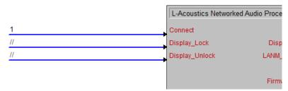
It is possible to use the standard "1" signal on all digital inputs of the module, especially on the **Connect** input. This will have the effect to instantly connect the module at program startup (for **Connect** input), or send the associated command as soon as the module connection is established (for other digital inputs).
